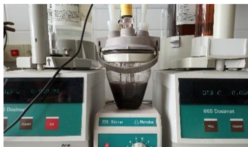
Fig. 2. System for potentiometric acid-base titration
