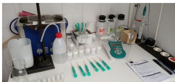
Fig. 3. System for sample pretreatment (sonicator and pH-meter)
